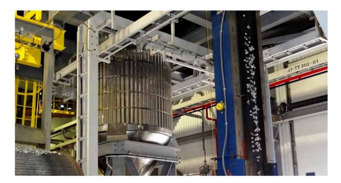
plywood and remanufacturing plants. IMT's magnetic separation solutions are being utilized extensively by these industry segments to protect and increase life of presses, grinders and chipping equipment from tramp metal contamination.
